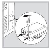
1 Open the terminal board by inserting a screwdriver into the side tabs of the cover. Use the screwdriver as a lever by pushing it down to open the cover (see diagram).
